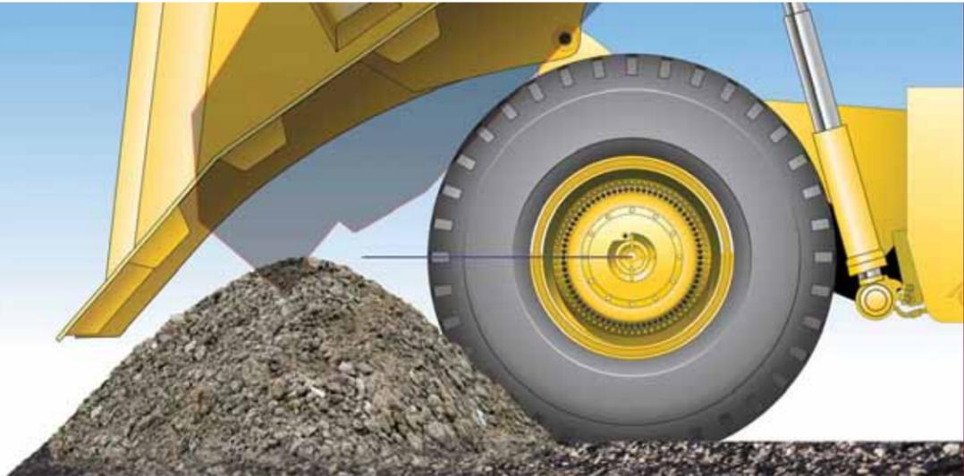
The (above) illustration compares the berm clearance between a typical OEM body (shadow) and the Westech Flow Control Body® (yellow body).
